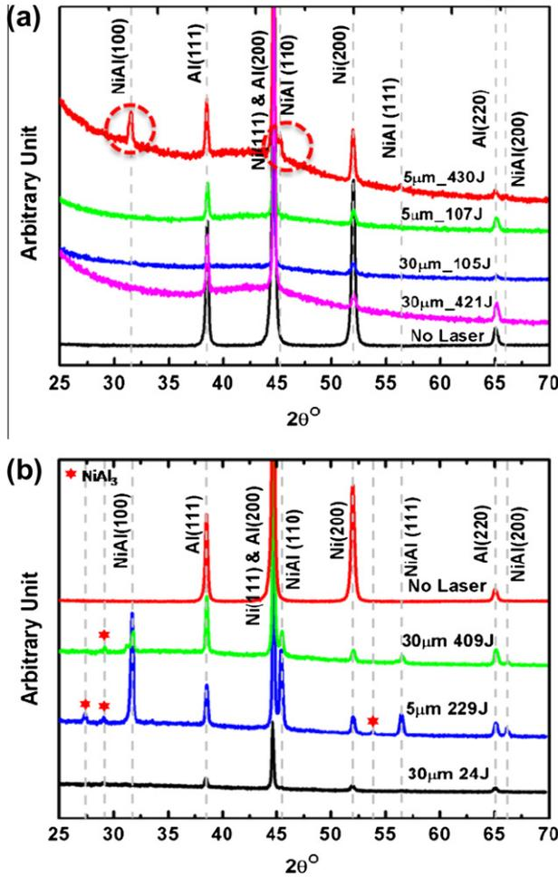
Fig. 9. X-ray diffraction of cross-sectional surfaces of (a) 3 ns and (b) 8 ns laser irradiation. (a) Reaction for 430 J irradiation (5  $\mu\text{m}$  bilayer), represented by circles. (b) Reaction from 229 to 409 J and both 5 and 30  $\mu\text{m}$  bilayer thickness.  $\text{NiAl}_3$  intermetallic compound was marked by stars.
