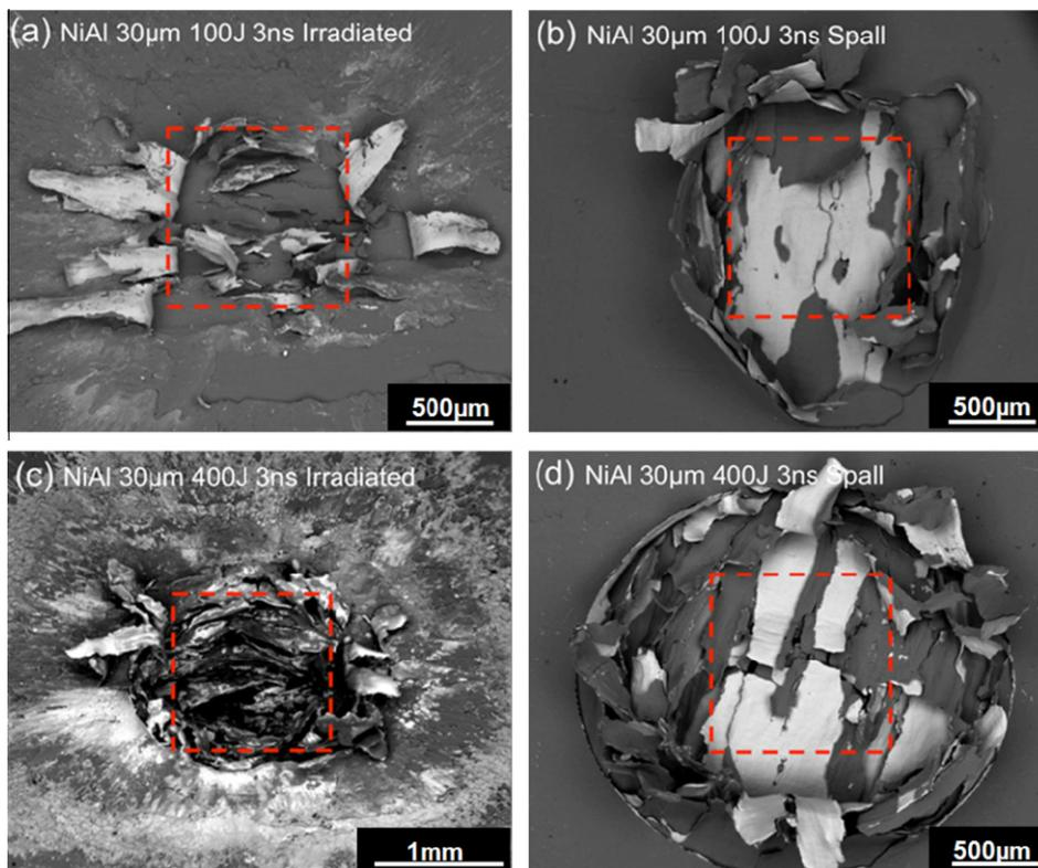
Fig. 5. SEM-BSE observations of samples with thicker bilayer (30  $\mu\text{m}$ ) exposed to (a and b) 100 J 3 ns and (c and d) 400 J 3 ns laser irradiation; (a and c) irradiated surface presenting melt, deposition from metal vaporization, and foil recoiling. Spall surfaces (b and d) revealed broken and peeled strips, without evidence of reaction.
