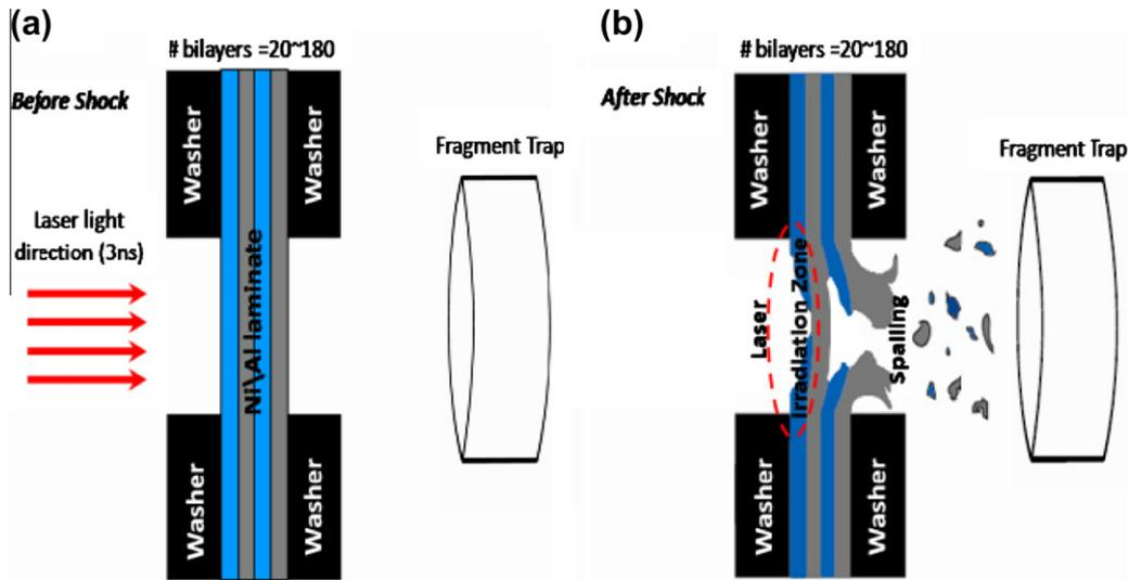
Fig. 2. Laser shock experimental setup: (a) sample placed between laser irradiation source and fragment trap, washers used to fix samples; (b) after laser irradiation, spall is formed and fragments are scattered from the spall surface and captured by fragment trap.
