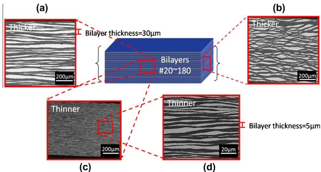
Fig. 1. Morphologies of sections of Ni–Al laminates (central schematic): (a) laminate with thicker (30  $\mu\text{m}$ ) bilayer; (b) laminate along longitudinal section; (c) laminate with thinner (5  $\mu\text{m}$ ) bilayer; (d) high magnification image of thinner bilayer.
