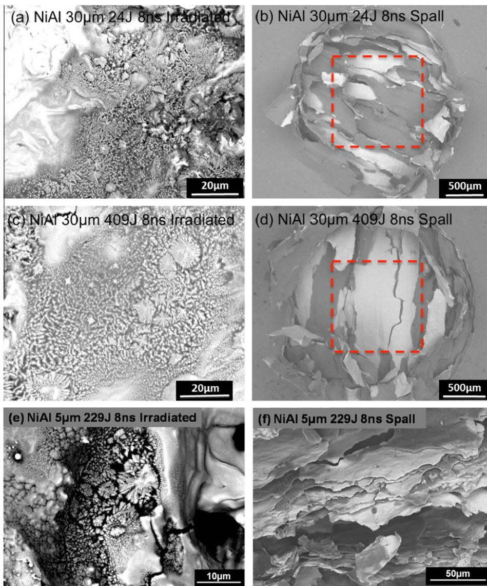
Fig. 7. 30  $\mu\text{m}$  bilayer laminates (8 ns pulse duration): (a) 24 J irradiated surface; (b) 24 J spall surface; (c) 409 J irradiated; (d) 409 J spall. Both irradiated surfaces show reactions but none of the spall surfaces have reactions. (e) Ni/Al laminates with 5  $\mu\text{m}$  bilayer subjected to 229 J, 8 ns laser pulse with 229 J: irradiated surface presents melts, dendrites, and granules. Clear evidence of reaction is shown. (f) no reaction on spall surface.
