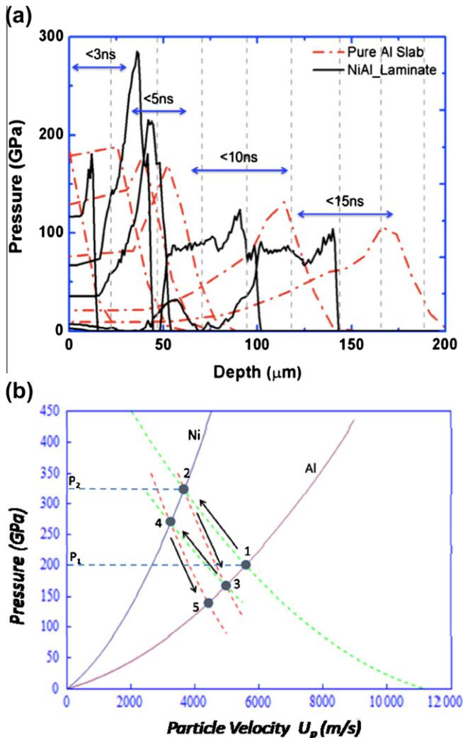
Fig. 3. Calculation of pressure pulse amplitude in Ni–Al: (a) laser shock wave (400 J; 3 ns) propagation in pure Al slab and laminate (HYADES Simulation); (b) Rankine–Hugoniot pressure vs. particle velocity plot for Ni and Al showing wave reflections.
