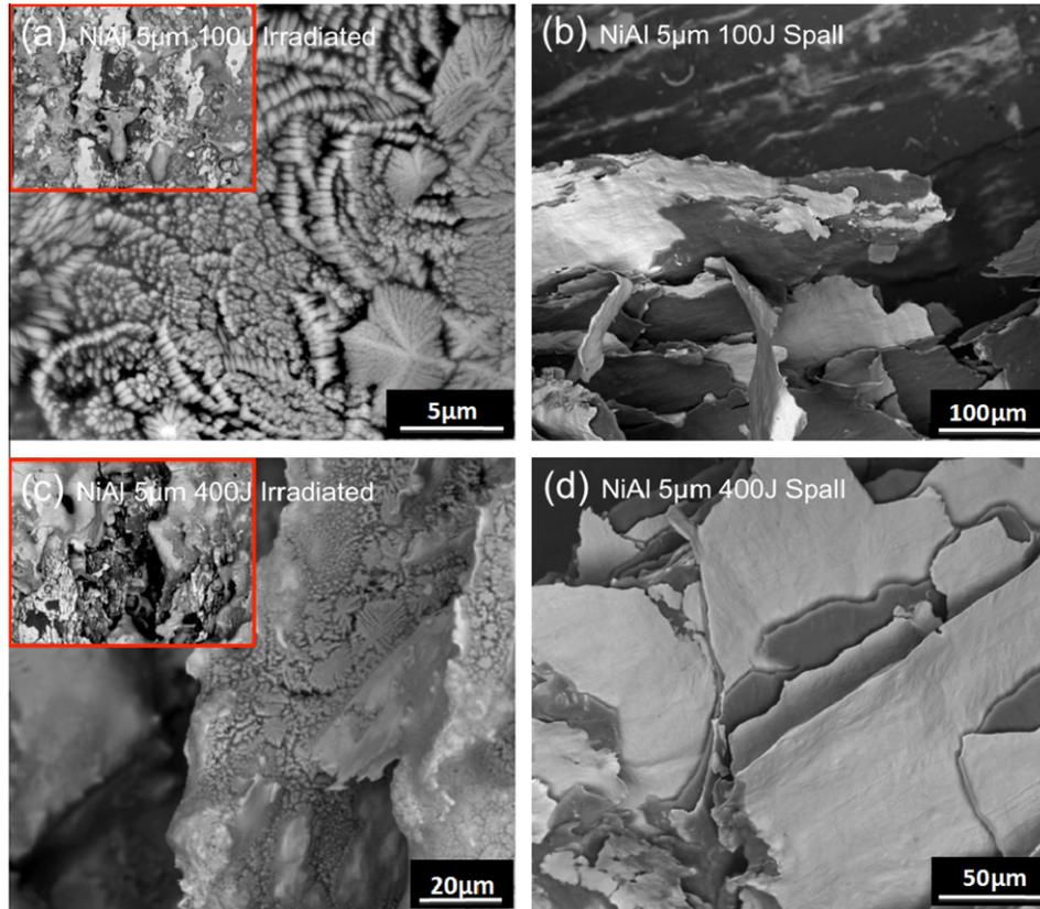
Fig. 6. SEM-BSE observations of samples with 5  $\mu\text{m}$  bilayer irradiated at (a and b) 100 J 3 ns and (c and d) 400 J 3 ns laser; (a and c) dendrites, melt pools, and granules found on the irradiated surface. Fractures (b and d) observed on spall surfaces.
