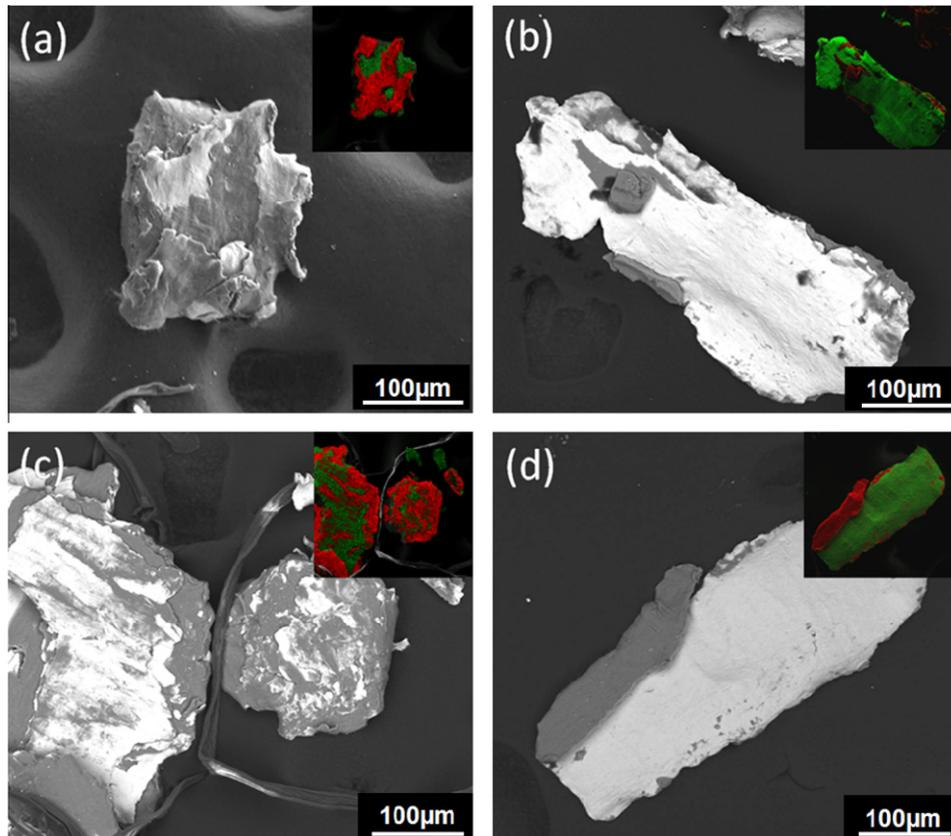
Fig. 4. Fragments from spall surface: (a) 5  $\mu\text{m}$  and (b) 30  $\mu\text{m}$  bilayer thickness (100 J 3 ns laser exposure); (c) 5  $\mu\text{m}$  and (d) 30  $\mu\text{m}$  bilayer thickness (400 J 3 ns laser exposure).
